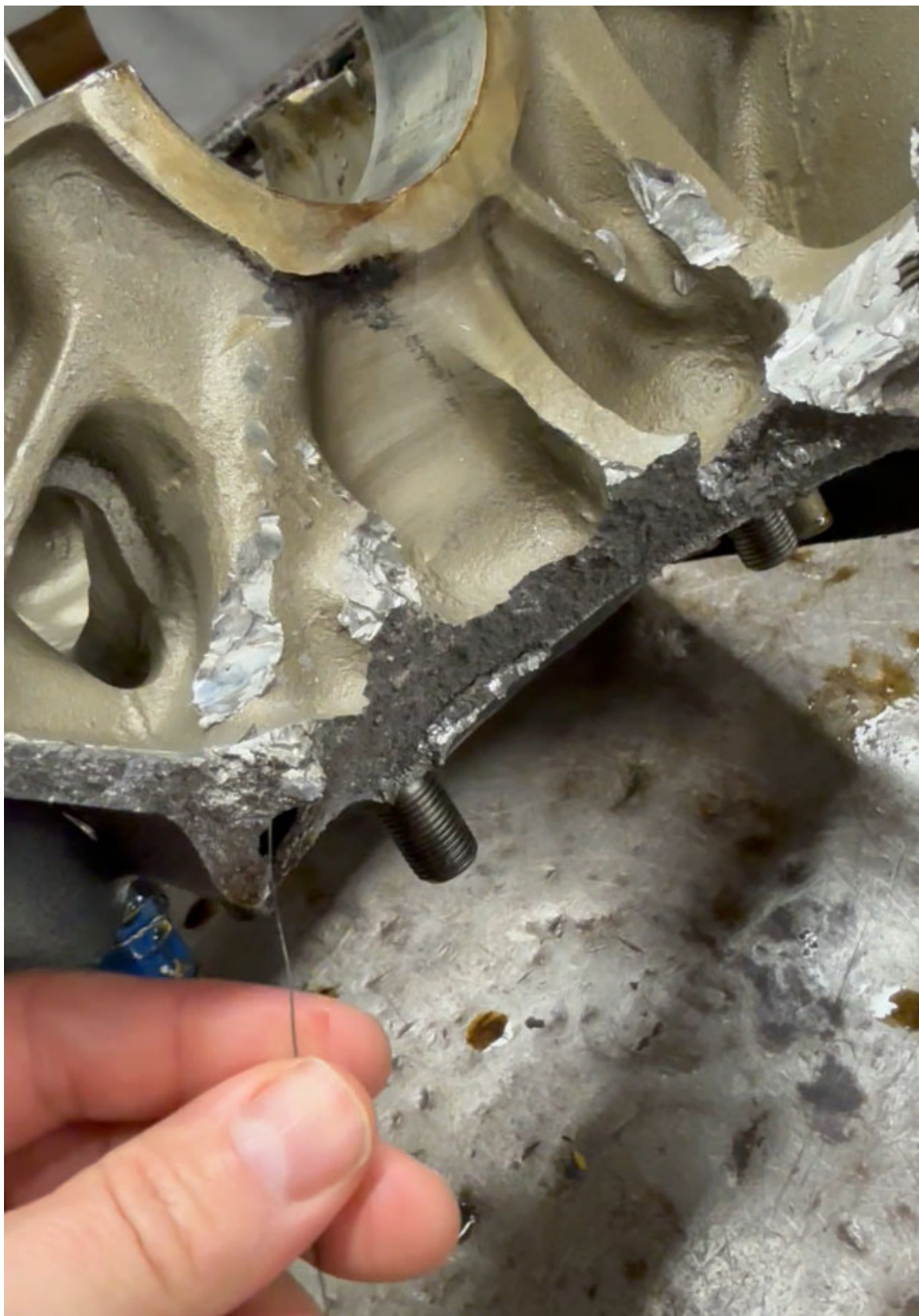
Figure 17: Oil passage found blocked
